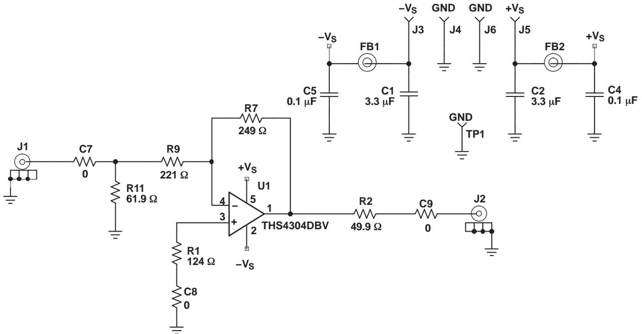
**Figure 43. Inverting Gain With Split Power Supply**
