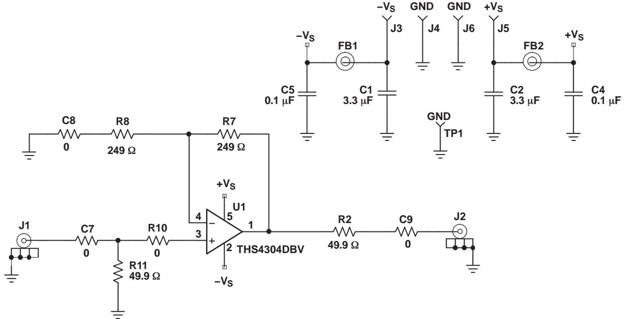
Figure 42. Non-Inverting Gain With Split Power Supply
