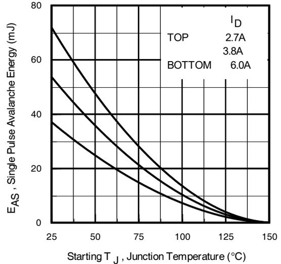
**Fig 14.** Maximum Avalanche Energy Vs. Drain Current
