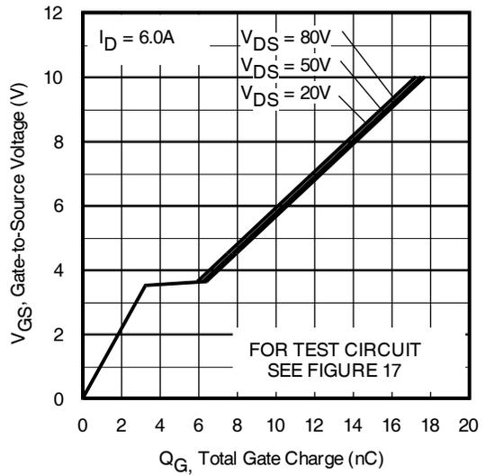
**Fig 10.** Typical Gate Charge Vs. Gate-to-Source Voltage
