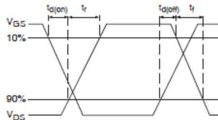
**Fig 14b.** Switching Time Waveforms
