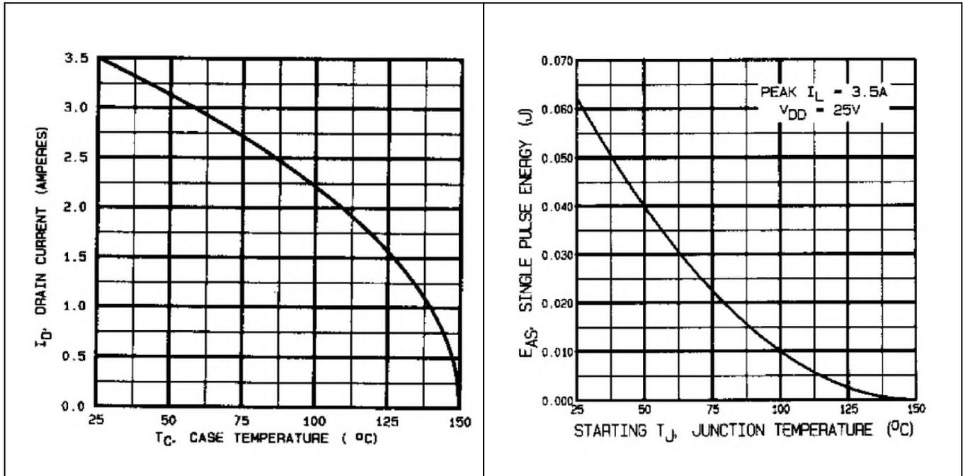
**Figure 9** Maximum Drain Current Vs. Case Temperature
