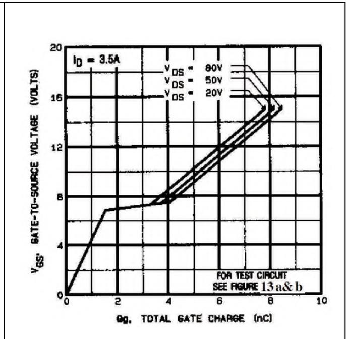
**Figure 6 Typical Gate Charge Vs. Gate-to-Source Voltage**
