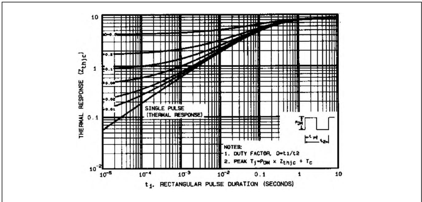
**Figure 11** Maximum Effective Transient Thermal Impedance, Junction-to-Case
