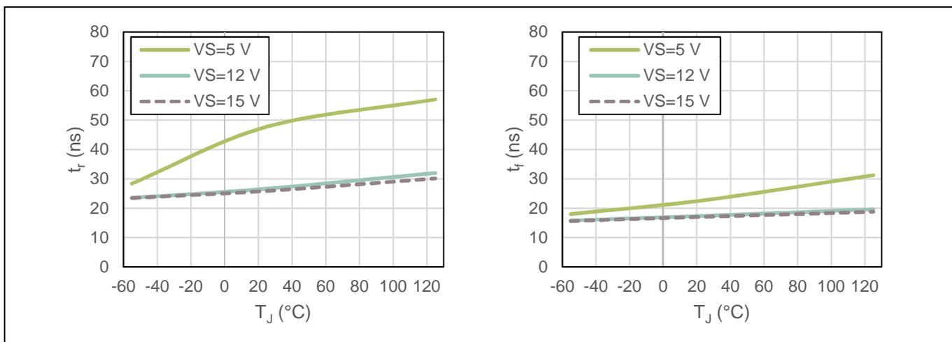
**Figure 11**  $t_f$  and  $t_r$  over temperature
