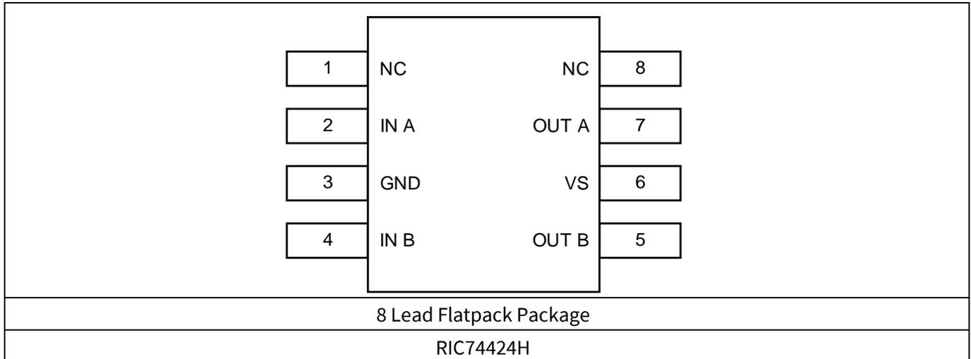
**Figure 3 RIC74424 pin assignments (top view)**
