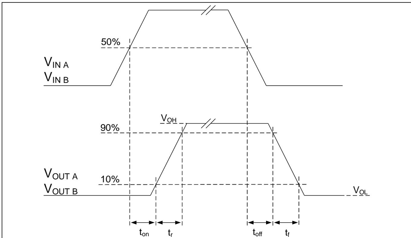
Figure 4 Propagation delay, rise and fall time definition
