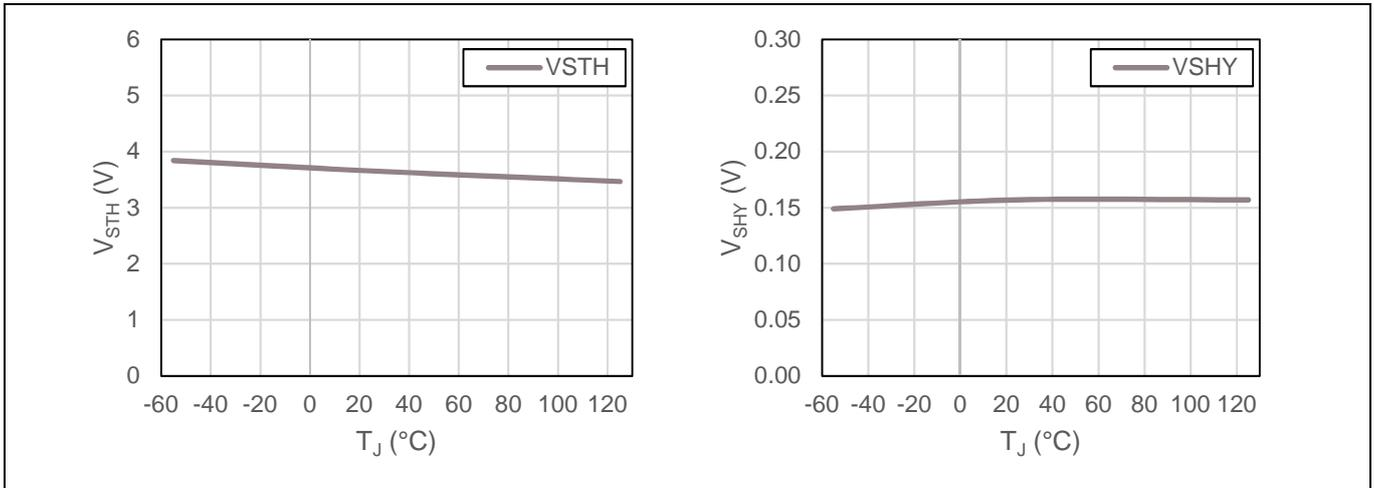
Figure 6 V<sub>STH</sub> and V<sub>SHY</sub> over temperature
