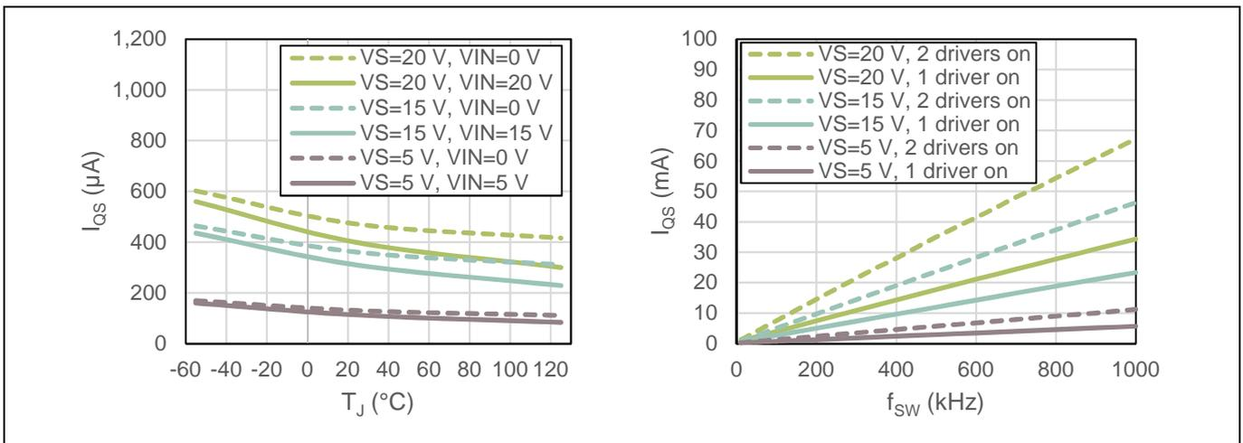
Figure 7 I<sub>QS</sub> over temperature and frequency
