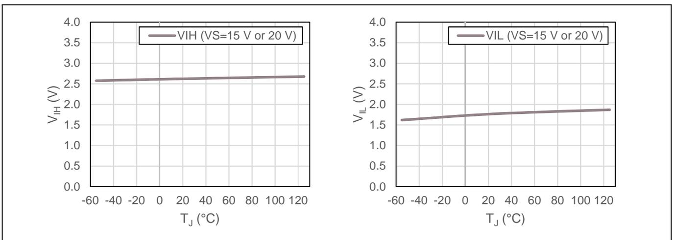
Figure 8 V<sub>IH</sub> and V<sub>IL</sub> over temperature
