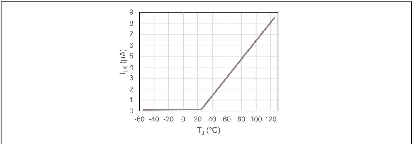
**Figure 12** I<sub>LK</sub> over temperature
