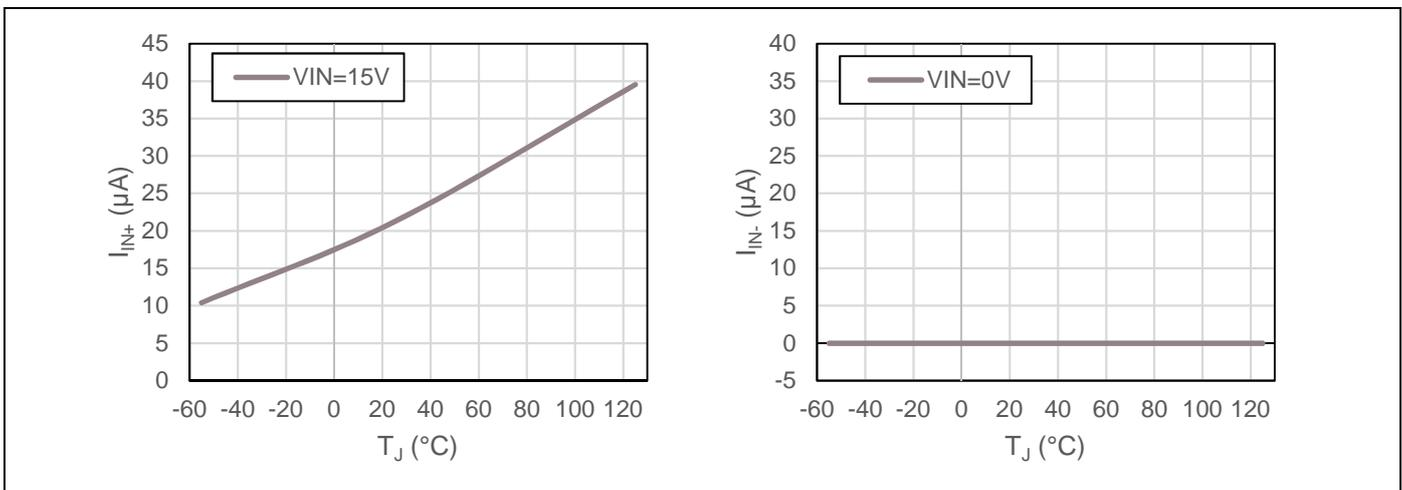
**Figure 14** I<sub>IN+</sub> and I<sub>IN-</sub> over temperature
