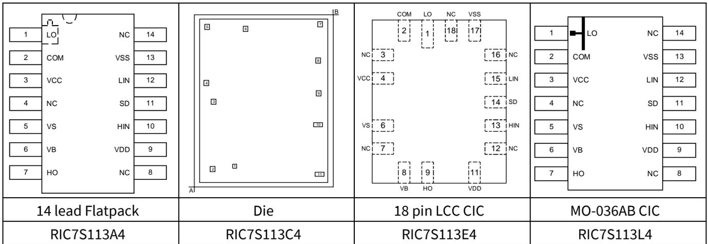
Figure 3 RIC7S113 pin assignments (top view)
