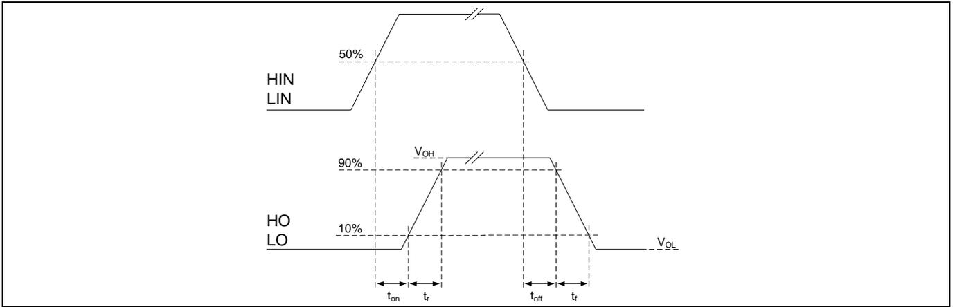
Figure 4 Propagation delay, rise and fall time definition
