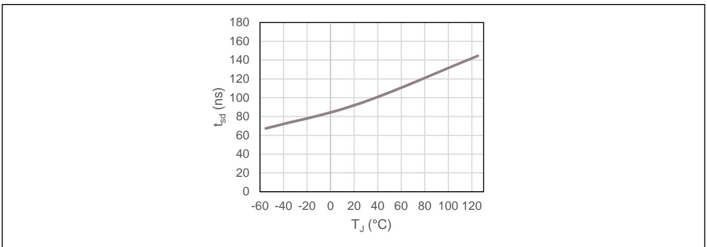
**Figure 17**  $t_{sd}$  over temperature
