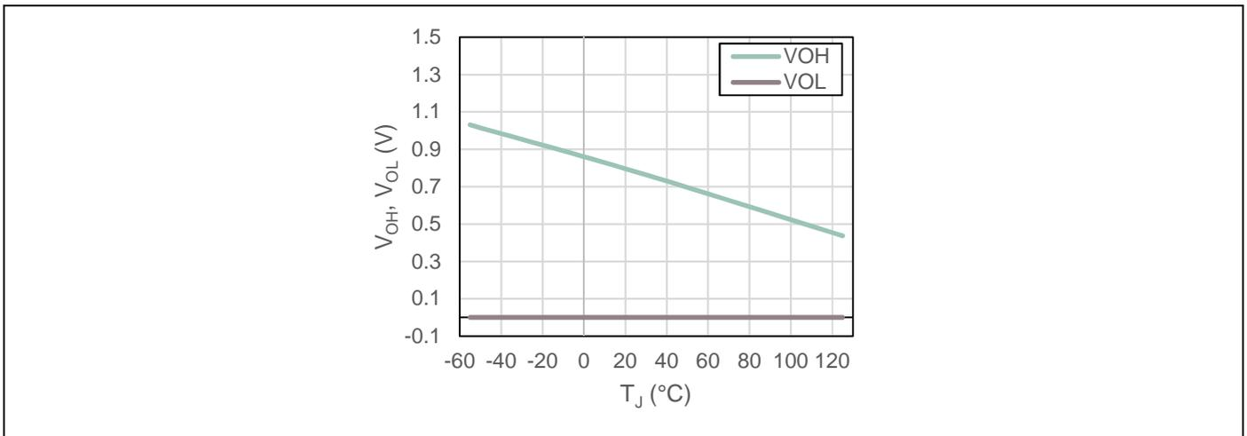
**Figure 15**  $V_{OH}$  and  $V_{OL}$  over temperature
