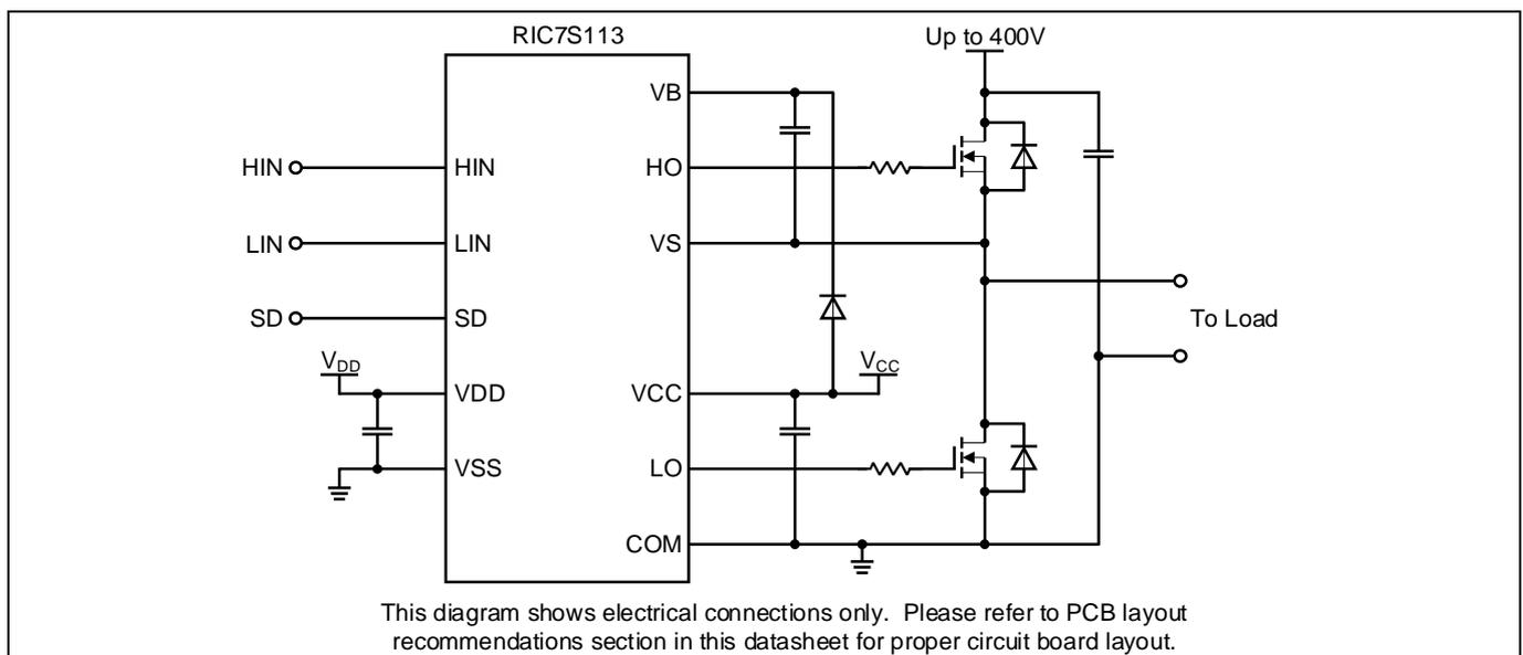
**Figure 1** Typical half bridge application block diagram
