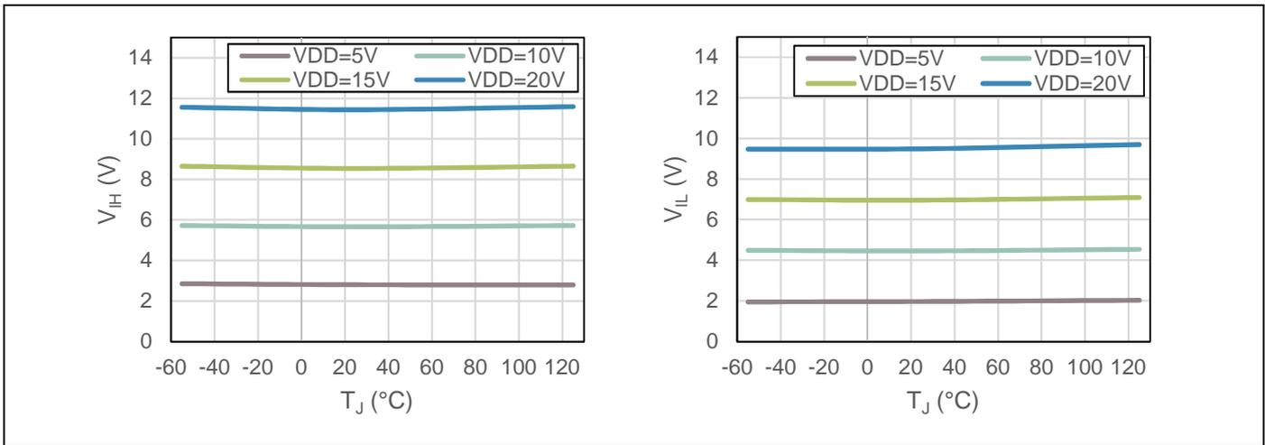
**Figure 13** V<sub>IH</sub> and V<sub>IL</sub> over temperature
