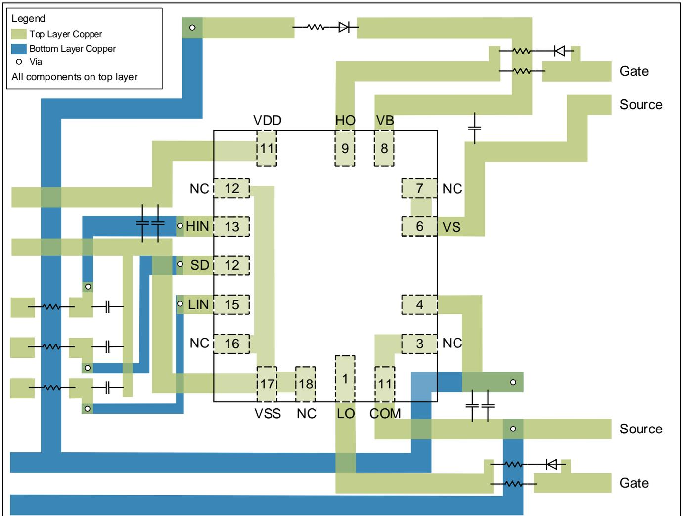
**Figure 25 Recommended PCB layout for RIC7S113E4 (LCC CIC)**
