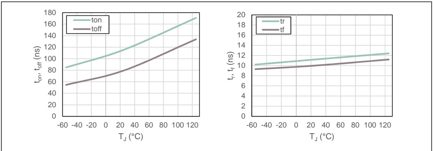
**Figure 16**  $t_{on}$ ,  $t_{off}$ ,  $t_r$  and  $t_f$  over temperature
