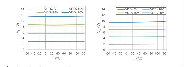
Figure 13  $V_{IH}$  and  $V_{IL}$  over temperature
