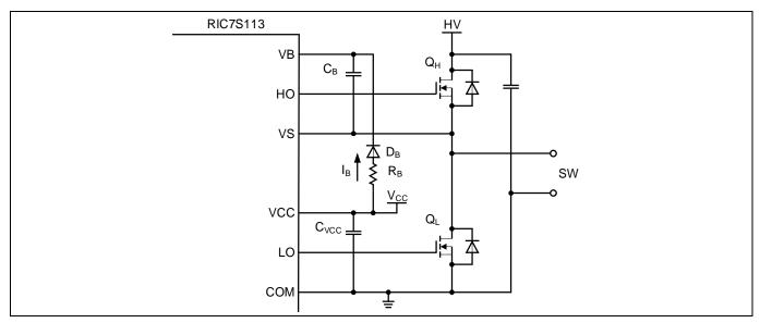
Figure 20 Example bootstrap circuit for high side bias power
