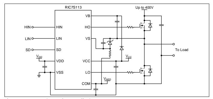
Figure 21 Example negative turn off voltage
