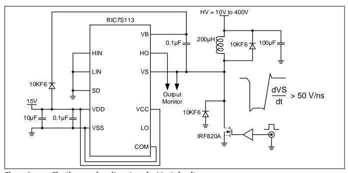
Figure 8 Floating supply voltage transient test circuit
