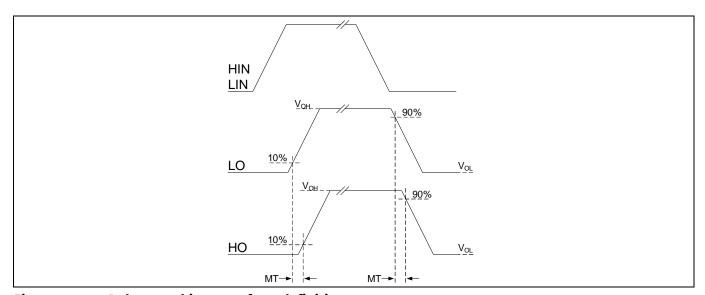
Figure 6 Delay matching waveform definitions
