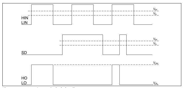
Figure 22 Input/output logic timing diagram
