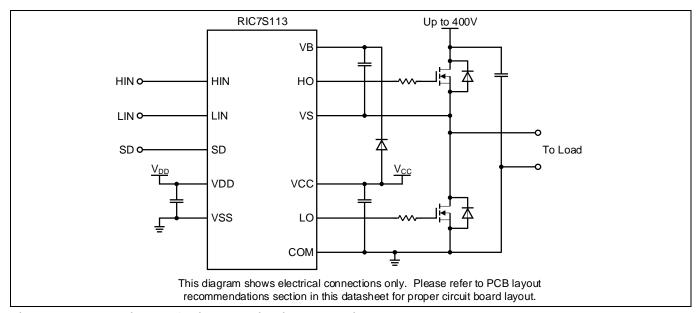
Figure 1 Typical half bridge application block diagram
