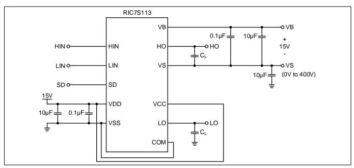
Figure 7 Switching time test circuit
