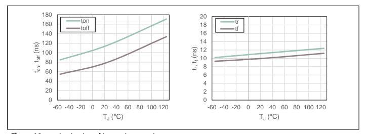
Figure 16  $t_{on}$ ,  $t_{off}$ ,  $t_r$  and  $t_f$  over temperature
