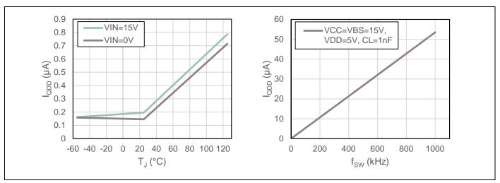
Figure 11 IQDD over temperature and frequency
