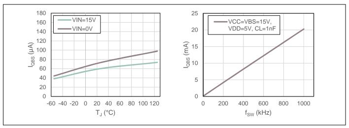
Figure 9 I<sub>QBS</sub> over temperature and frequency
