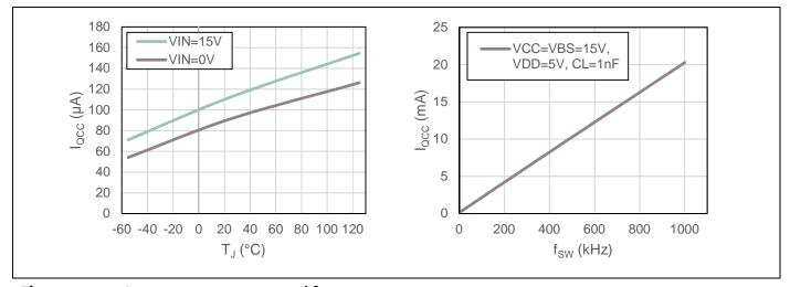
Figure 10 l<sub>QCC</sub> over temperature and frequency
