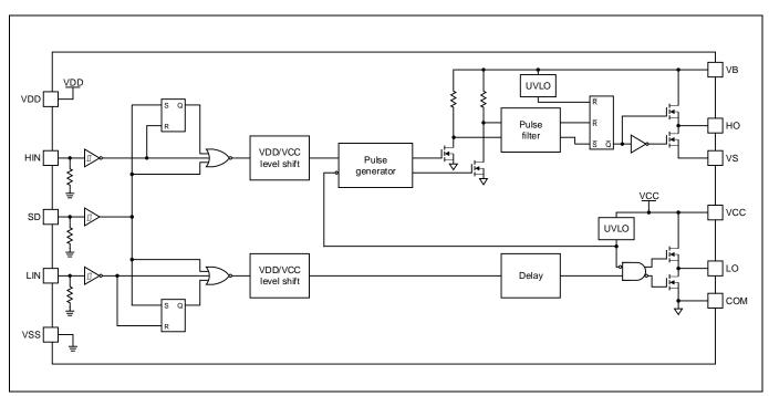
Figure 2 Block diagram
