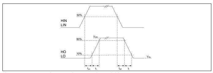
Figure 4 Propagation delay, rise and fall time definition
