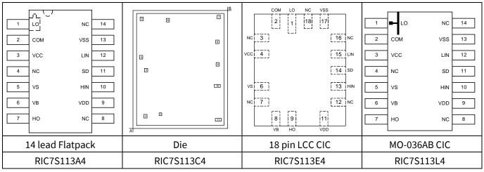
Figure 3 RIC7S113 pin assignments (top view)
