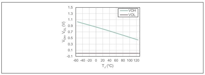
Figure 15  $V_{\text{OH}}$  and  $V_{\text{OL}}$  over temperature
