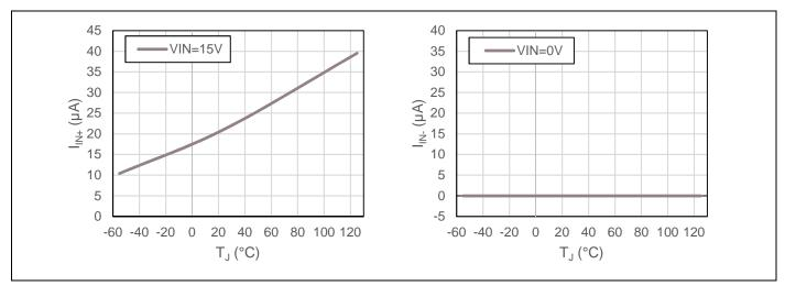
Figure 14 I<sub>IN+</sub> and I<sub>IN-</sub> over temperature
