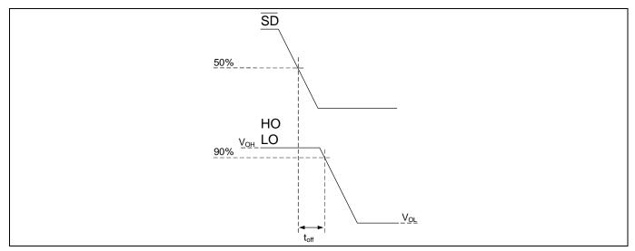
Figure 5 Shutdown waveform definitions
