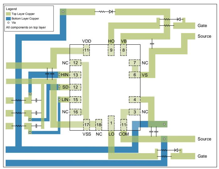
Figure 25 Recommended PCB layout for RIC7S113E4 (LCC CIC)
