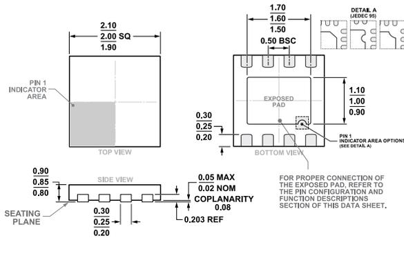
**Figure 3. 8-Lead Lead Frame Chip Scale Package [LFCSP]
