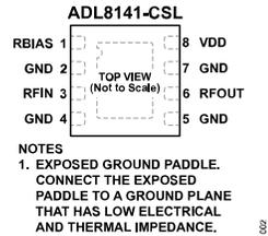
Figure 2. Pin Configuration
