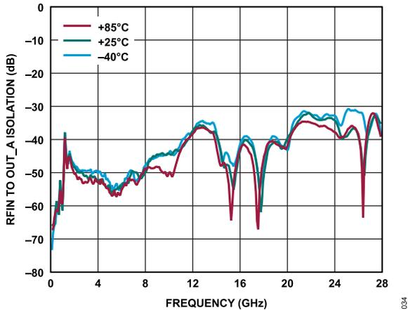
Figure 38. RFIN to OUT\_A Isolation vs. Frequency Over Temperature, 100 MHz to 28 GHz,  $V_{DD} = 8.5\text{ V}$ ,  $I_{DQ} = 90\text{ mA}$ , Mode = Internal Amplifier
