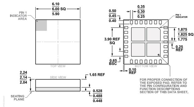
Figure 85. 28-Terminal Land Grid Array [LGA] (CC-28-4)
