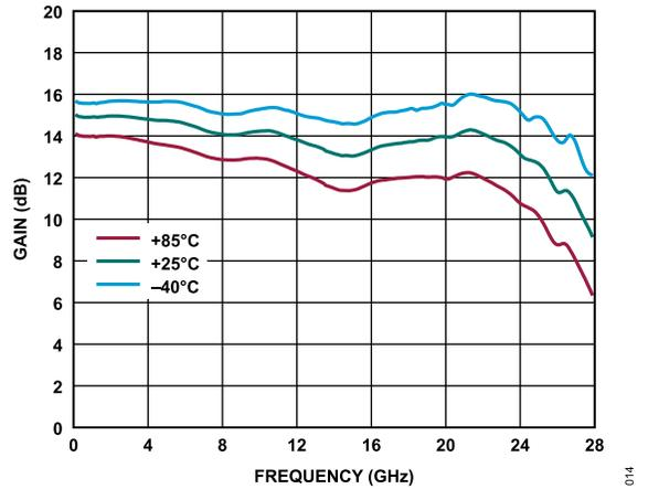
Figure 16. Gain vs. Frequency Over Temperature, 200 MHz to 28 GHz,  $V_{DD} = 8.5$  V,  $I_{DQ} = 90$  mA, Mode = Internal Amplifier
