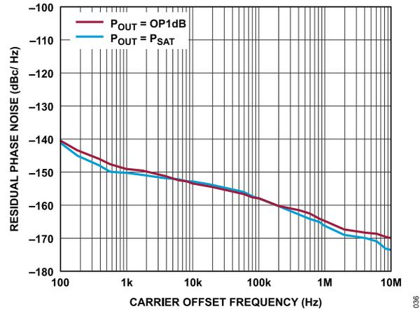
Figure 41. Phase Noise at 5 GHz
