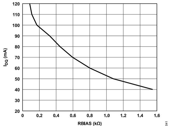
Figure 17.  $I_{DQ}$  vs.  $R_{BIAS}$ ,  $V_{DD} = 8.5$  V
