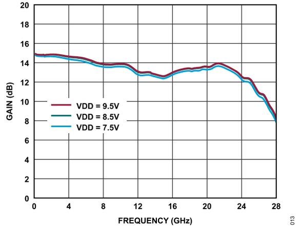
Figure 15. Gain vs. Frequency Over  $V_{DD}$ ,  $I_{DQ} = 90$  mA, 100 MHz to 28 GHz, Mode = Internal Amplifier
