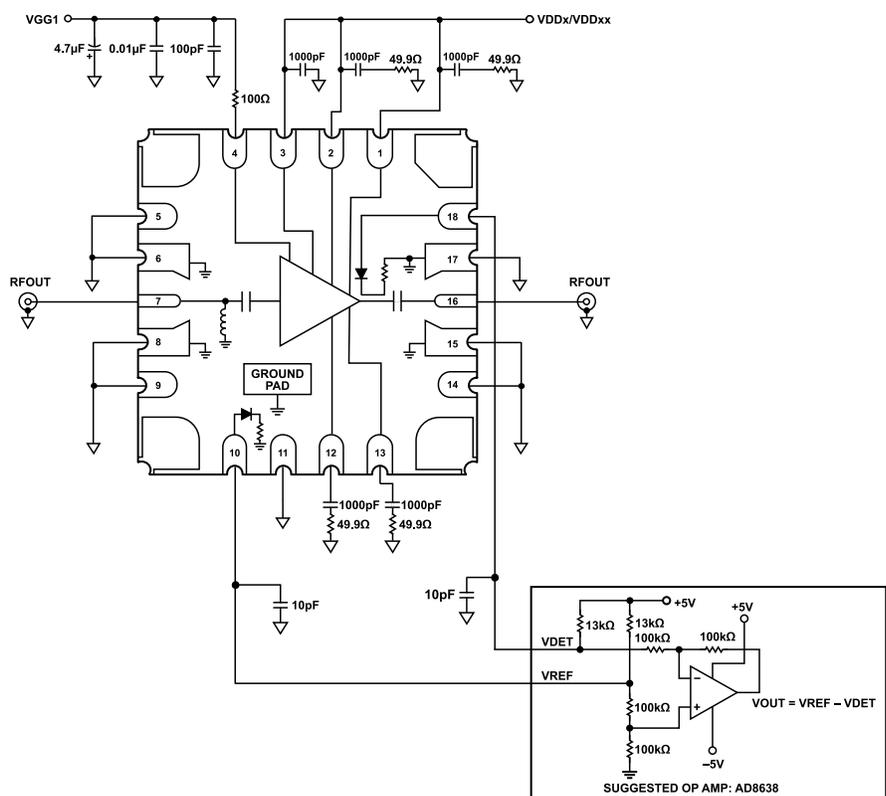
Figure 47. Basic Connections
