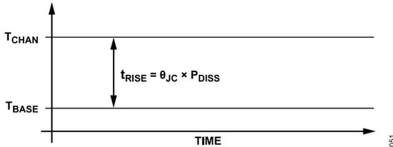
Figure 48. Channel Temperature Rise for Continuous Bias Condition
