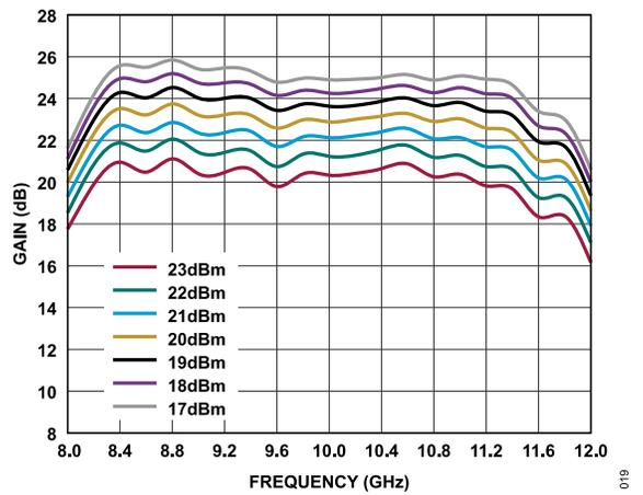
Figure 20. Gain vs. Frequency for Various  $P_{IN}$  Levels
