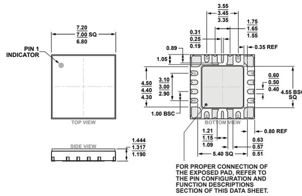
Figure 50. 18-Terminal Ceramic Leadless Chip Carrier with Heat Sink [LCC\_HS] (EH-18-1)
