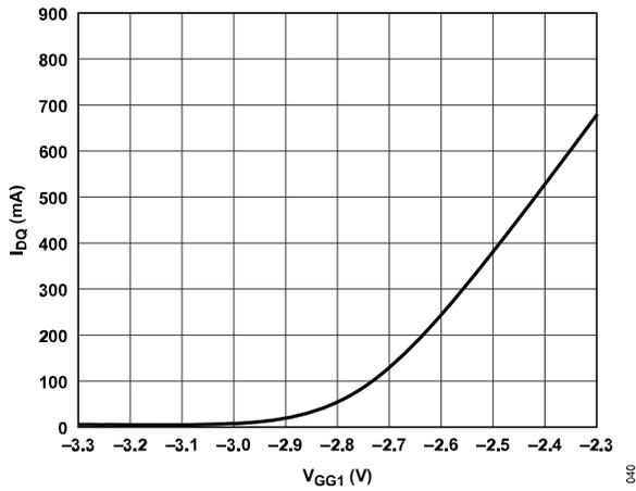
Figure 29.  $I_{DQ}$  vs.  $V_{GG1}$ ,  $V_{DD} = 28$  V
