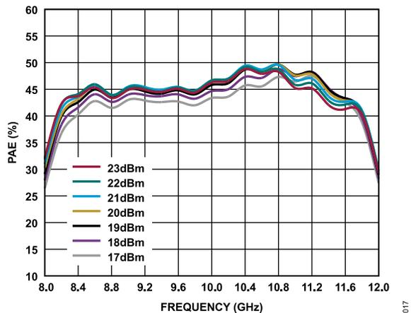
Figure 24. PAE vs. Frequency for Various  $P_{IN}$  Levels
