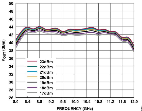
Figure 18.  $P_{OUT}$  vs. Frequency for Various  $P_{IN}$  Levels
