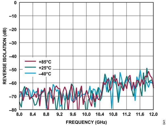
Figure 28. Reverse Isolation vs. Frequency for Various Temperatures
