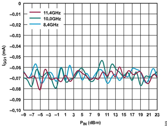
Figure 30.  $I_{GG1}$  vs.  $P_{IN}$  for Various Frequencies
