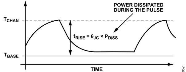
Figure 49. Pulsed Bias at Low Duty Cycle
