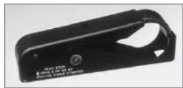
2-Step Cable Stripper with self-adjusting replacement blades for RG-6, 58, 59 & 62.
