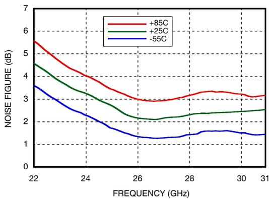
**Noise Figure vs. Temperature @ Vdd = +5V**
