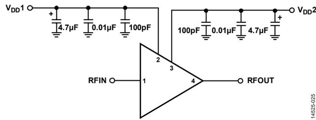
Figure 23. Typical Application Circuit with Self Biased Option
