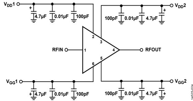
Figure 22. Typical Application Circuit with Gate Control Option
