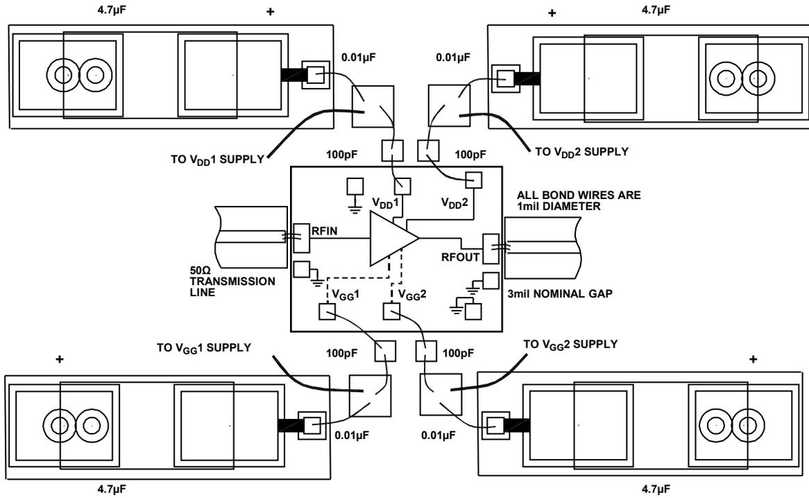
Figure 24. Assembly Diagram with Gate Control Option
