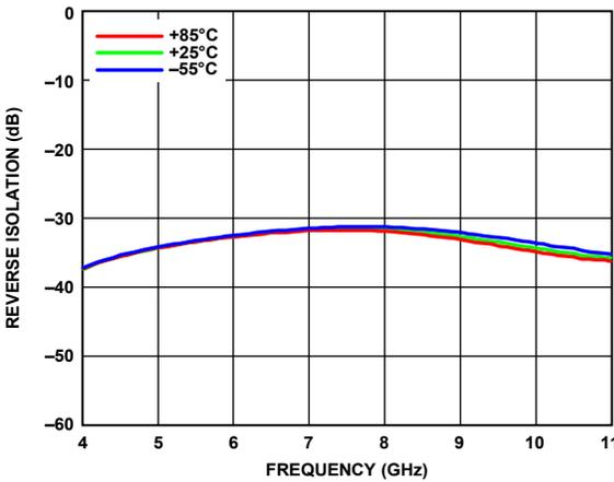
Figure 15. Reverse Isolation vs. Frequency at Various Temperatures
