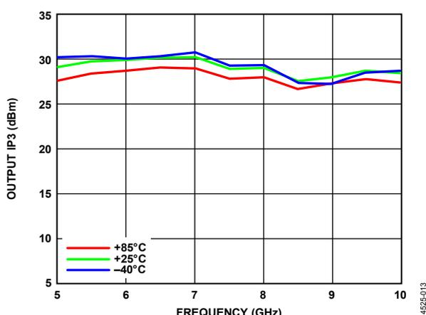
Figure 13. Output IP3 vs. Frequency at Various Temperatures
