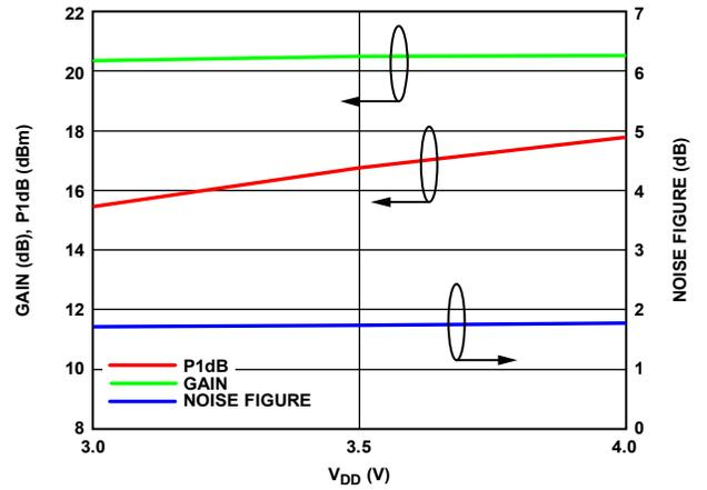
Figure 18. Gain, P1dB, and Noise Figure vs. Supply Voltage (V<sub>DD</sub>) at 7 GHz
