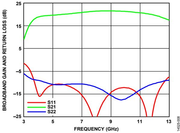
Figure 8. Broadband Gain and Return Loss vs. Frequency
