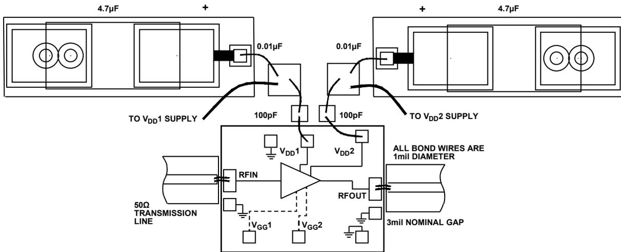
Figure 25. Assembly Diagram with Self Biased Option
