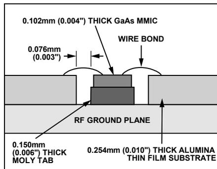
Figure 21. Routing RF Signal with Moly Tab
