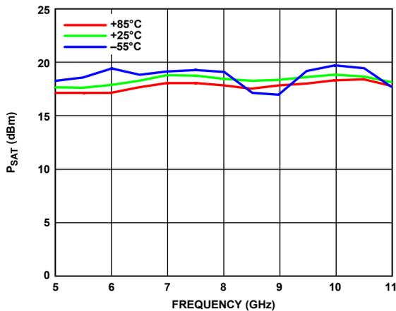
Figure 16. P<sub>SAT</sub> vs. Frequency at Various Temperatures
