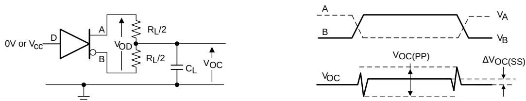
图 12. Measurement of Driver Differential and Common-Mode Output With RS-485 Load
