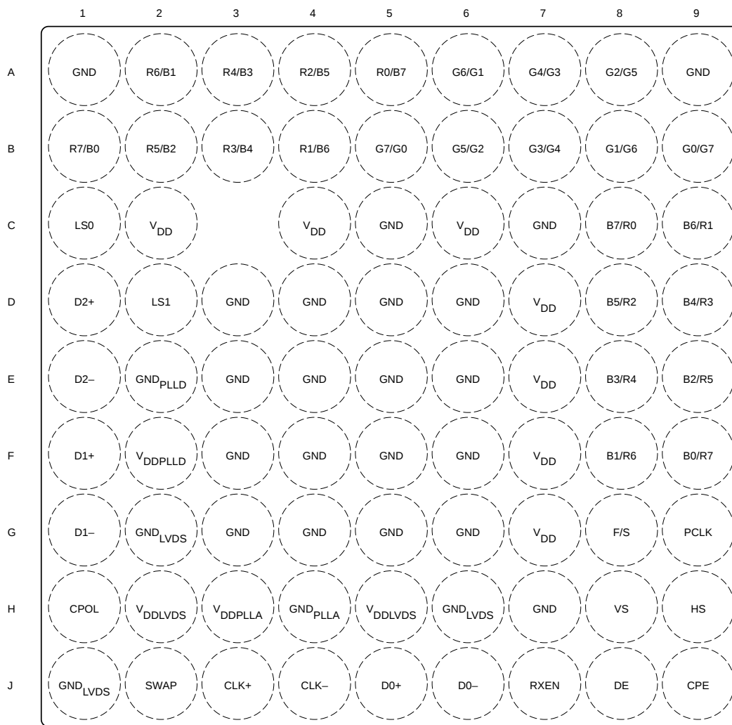
图 5-1. ZXH Package 80-Pin nFBGA Top View
