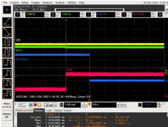
Figure 3. OC_FLAGB Response Time (Toggle R_{LOAD} from High to Low Resistance)
