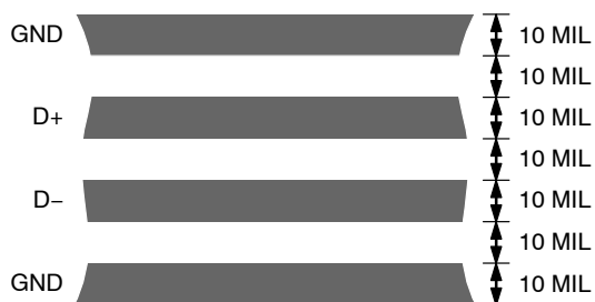
Figure 22. Arrangement of Signal Tracks
