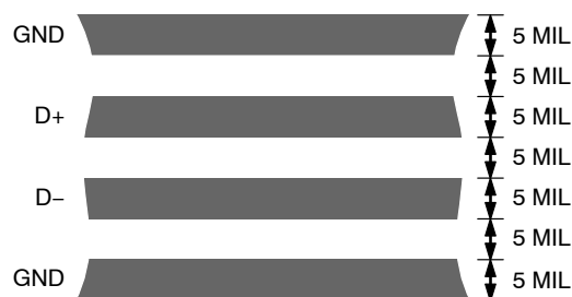
Figure 22. Typical Arrangement of Signal Tracks
