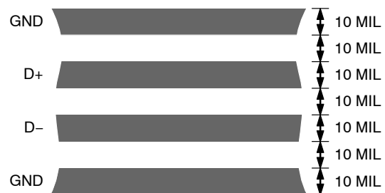
Figure 17. Arrangement of Signal Tracks
