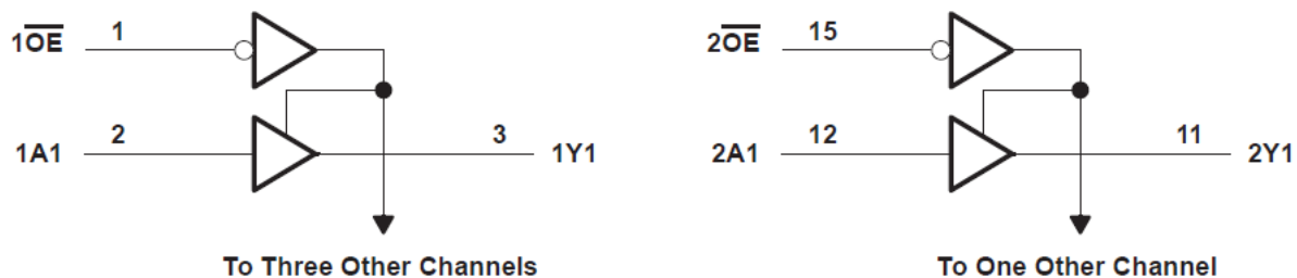
图 8-1. Logic Diagram (Positive Logic)
