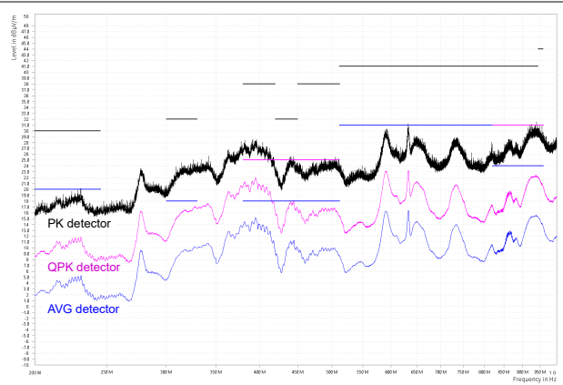
图 9-19. CISPR 25 Class 5 Radiated EMI, Log Antenna, Vertical Polarization, 200 MHz to 1 GHz
