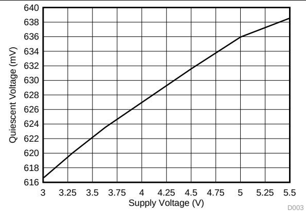
图 2. Quiescent Voltage vs Supply Voltage
