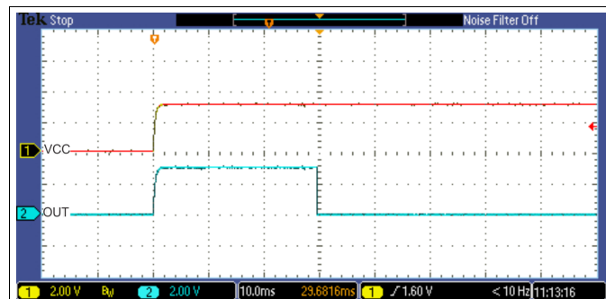
Figure 14. TMP303A Power-On Response, T_A Less Than 60°C
