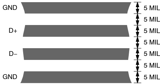
Figure 21. Typical Arrangement of Signal Tracks
