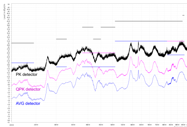
图 8-20. CISPR 25 Class 5 Radiated EMI, Log Antenna, Vertical Polarization, 200MHz to 1GHz
