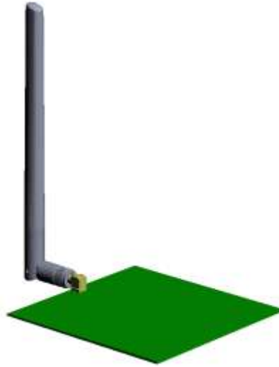
Figure 11. On edge of ground plane, Bent 90 Degrees
